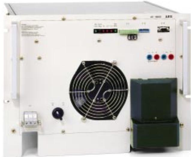
Transistors create an AC voltage of 80 kHz from it. Transfer devices are used for electrical isolation as well as adaptation of the voltage to the secondary side. After this, the high-frequency AC voltage is rectified using fast diodes. An output filter is installed in order to reduce the voltage ripple. The output voltage and the output current are controlled by pulse width modulation of the transistor switch on the primary side.
