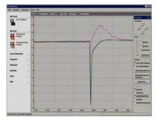
Free BACS<sup>®</sup> viewer software shows the Equalization (Balancing) of a battery (the bold violet line in the graphic) within a string of 32 batteries during a discharge/recharging process. BACS<sup>®</sup> Equalization (Balancing) prevents the overcharging of the violet battery, while the batteries around it continue to charge.
