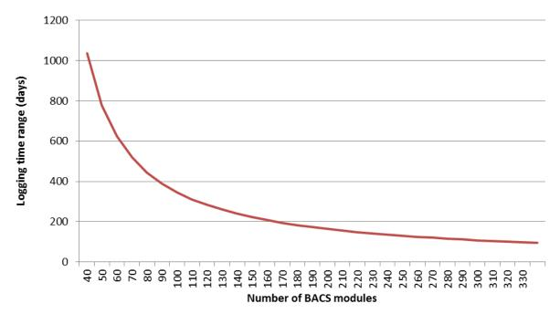
Flash ROM capacity for battery history depending on no. of BACS<sup>®</sup> modules in the system
