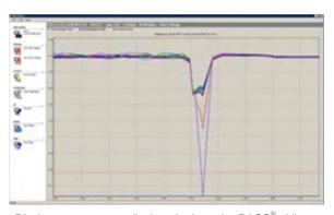
Discharge process displayed through BACS<sup>®</sup> Viewer software shows the voltage drop of several batteries during a discharge, unnoticed by the UPS. In a later stage, these accumulators would cause the complete system to collapse! BACS<sup>®</sup> corrects this problem and attempts to fully recharge this specific battery.
