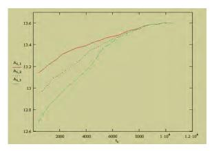
Oscilloscope graph of battery voltages during the Equalizing (Balancing) process: The voltages of the 3 batteries behave differently given the regulating influence of the BACS<sup>®</sup> modules. The ideal harmonic charging curve will be achieved for every battery in the string.
