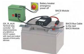
The GX\_R\_AUX module provides 4 relay contacts and 4 digital inputs. It controls up to 4 breakers. The digital inputs read the battery breaker status and display it in the BACS<sup>®</sup> web interface. Other alarm devices (for example, audio alarms) may be connected to the outputs or digital inputs of the GX\_R\_AUX.
