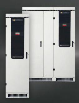
The Protect RCS DC system has been developed and designed to provide high reliability power supply and battery charging capability. The Protect RCS DC system is a thyristor-controlled rectifier suitable for charging nickel-cadmium or lead-acid batteries while supplying DC loads. It can also be used without batteries as a direct power supply.
