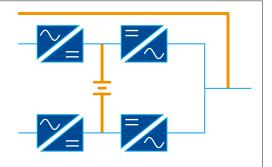
A central static bypass switch is fitted, sized for the whole UPS power and a single battery bank is connected to the UPS.
